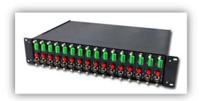
2U chassis of video digital optical converter is a kind of standard chassis, which could meet the users' demand of concentration and centralized management.
